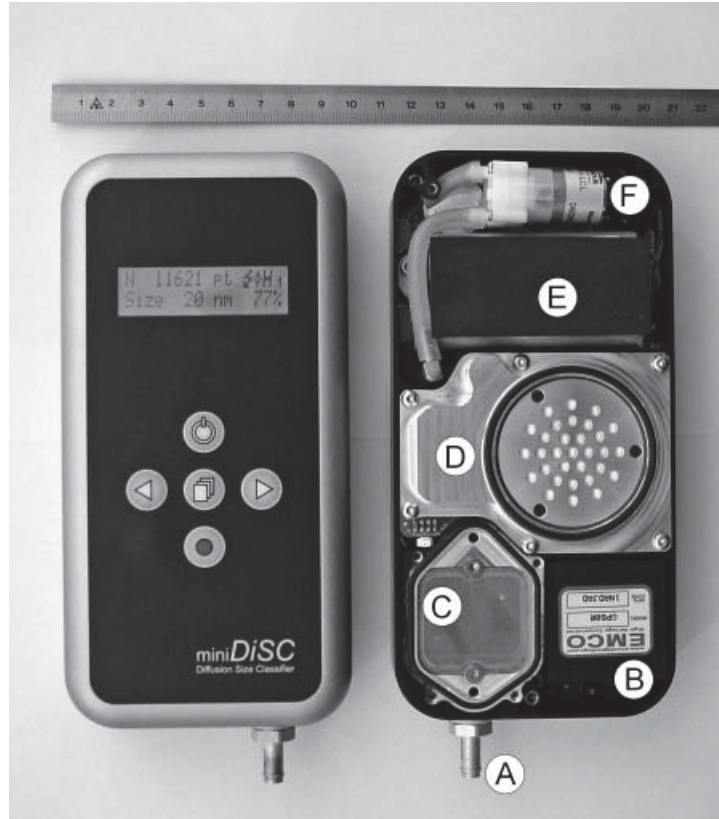
Figure 1-5. The miniature DiSC, front (left), and opened back (right) [28]
